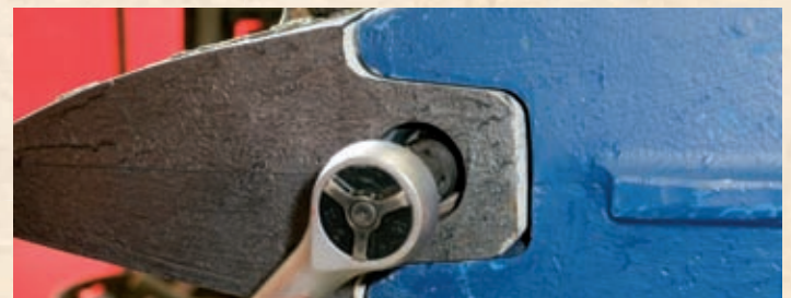
One-tool locking with Tufflock™
